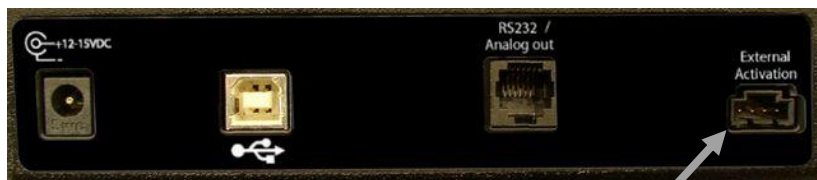
Figure 35: External Activation Switch input
