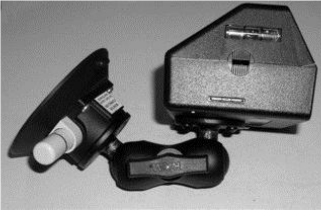
Figure 4: Assembly w/single vacuum cup
